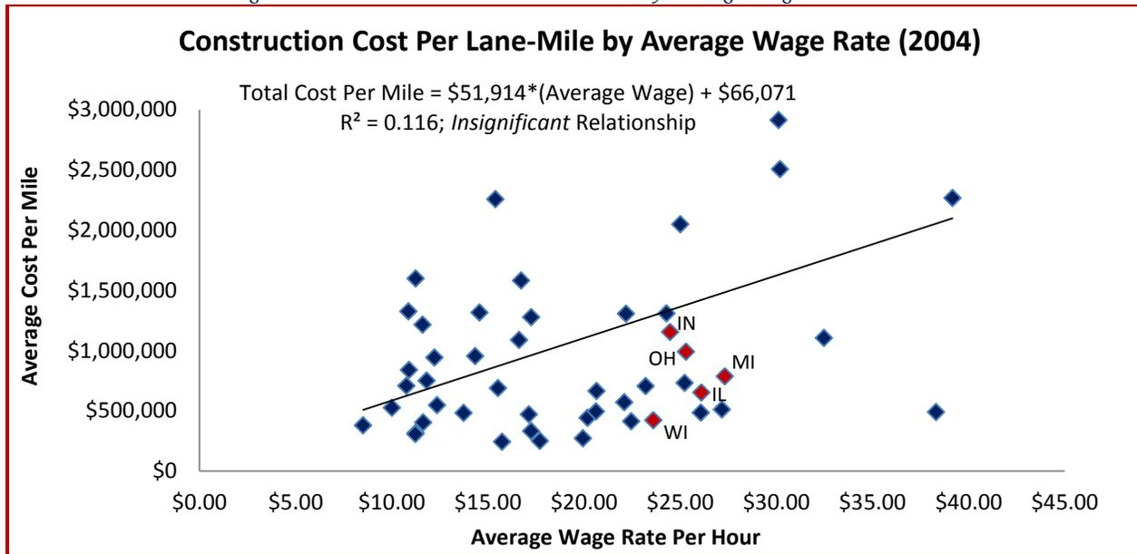
Source(s): Poupore (2004), "The Impact of Wages on Highway Construction Costs: Updated Analysis," The Construction Labor Research Council.
